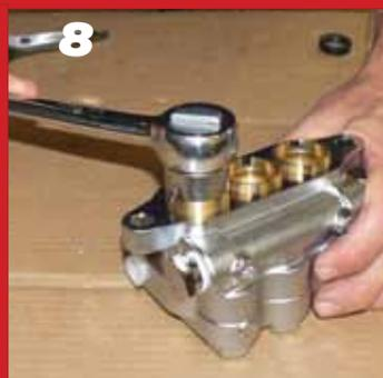
8 Remove Seal Case from each seal chamber. Remove O-Ring from outside diameter of Seal Case.
