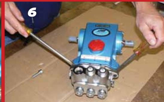
6 Separate Manifold Head from crankcase by turning the shaft, insert 2 screwdrivers in gap and pry Manifold Head forward until it comes off.
